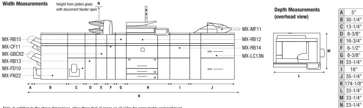
Note: In addition to the above dimensions, allow three feet of space on all sides for consumable replenishment, paper jam removal, and maintenance and service procedures. Images may not be to scale.
